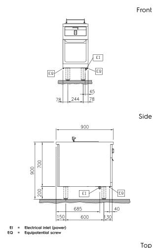
Electric Supply voltage: 400 V/3N ph/50/60 Hz Total Watts: 10 kW **Key Information:** Number of wells: Usable well dimensions (width): 240 mm Usable well dimensions 225 mm (height): Usable well dimensions 380 mm (depth): Well capacity: 12 lt MIN; 14 lt MAX Thermostat Range: 100 °C MIN; 180 °C MAX External dimensions, Width: 400 mm External dimensions, Depth: 900 mm External dimensions, Height: 700 mm Net weight: 75 kg On Base;One-Side Configuration: Operated Sustainability
